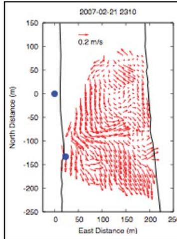
These one-dimensional velocity map outputs from a RiverSonde can be combined with those from additional RiverSondes to create continuous realtime two-dimensional vector maps of surface current velocity and direction, in similar manner as SeaSonde, but on a smaller scale (spatially and temporally). Synoptic measurement of 2D velocity distributions in river flows such as this is not possible using any other technology.
