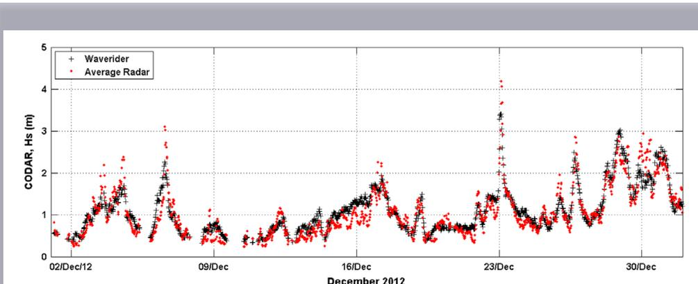
*Adjacent Figure: Time series of significant waveheight (Hs) during December 2012 generated by a 25 MHz CODAR SeaSonde (red points) against waverider buoy Hs (black points). From Atan, R., J. Goggins, M. Harnett, P. Agostinho, and S. Nash. "Assessment of Wave Characteristics and Resource Variability at a 1/4-Scale Wave Energy Test Site in Galway Bay Using Waverider and High Frequency Radar (CODAR) Data." Ocean Engineering, Vol. 117, 272-291 (2016).*
