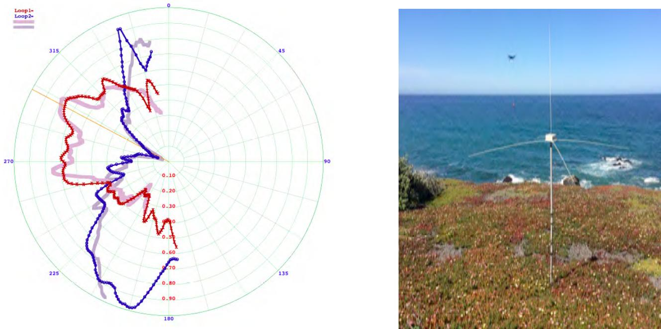
Figure 1: Antenna pattern from drone in red and blue plotted overtop transponder pattern (left) and drone flying in front of SeaSonde receive antenna (right).
