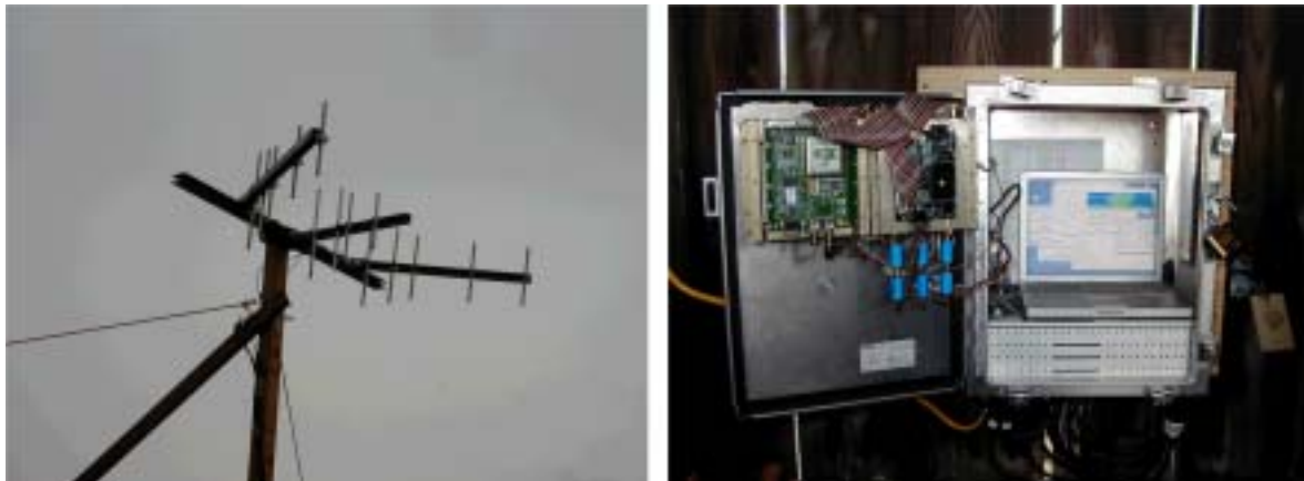
Fig. 1 (a) RiverSonde Antenna. Energy is Transmitted on the Center Yagi and Received on all 3 Yagis. (b) River Sonde Equipment and Laptop Computer. The Weather-resistant Enclosure is Installed Inside a Storage Building
