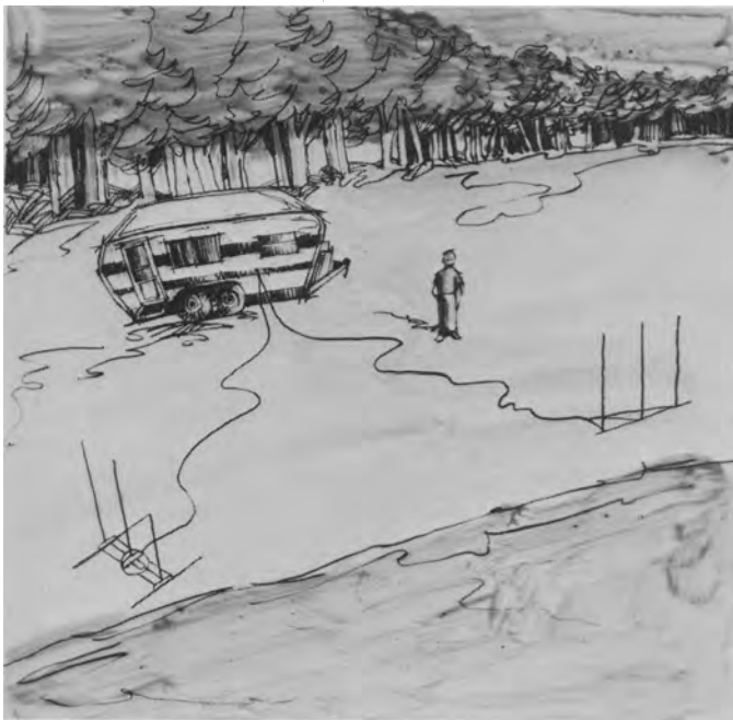
Fig. 2 (left). Sketch of the system as operated on the beach. Transmitting antennas are on the left and receiving antenna on the right. Fig. 3 (right). Block diagram of radar system.
